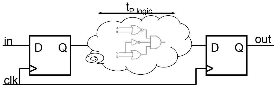
$$t_{\text{Critical}} = t_{P \text{ FF}} + t_{P \text{ logic}} + t_{S \text{ FF}}$$
