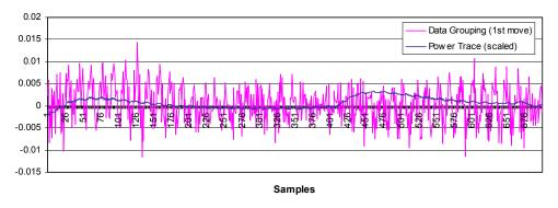
Figure 6. Differential Power Analysis - Data Grouping
