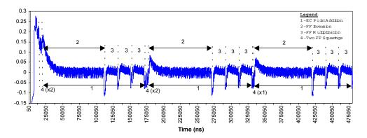
Figure 1. τ-adic Point Multiplication Power Trace (k=0x2B)
