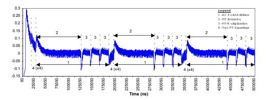
**Figure 2.** τ-adic Point Multiplication with Windowing Power Trace (k=0x53E4)
