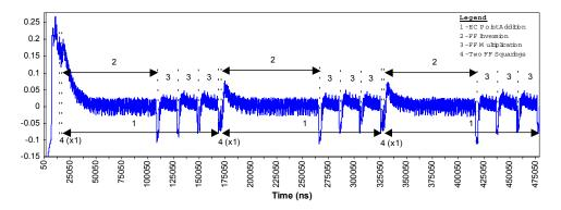
Figure 4. Koblitz Curve Specific DPA Countermeasure 2 (Algorithm 3) Power Trace (k=0xB)
