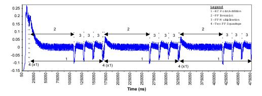
**Figure 3.** SPA Resistant Point Multiplication (Algorithm 1) Power Trace (k=0xA)
