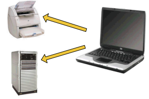
Figure 6: One-to-many communication, e.g. laptop has access to network resources (fixed backbone) via access point.
