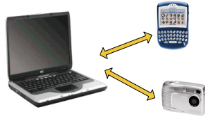
Figure 2: Many-to-one communication, e.g. a PAN with many consumer devices talking to a laptop.
