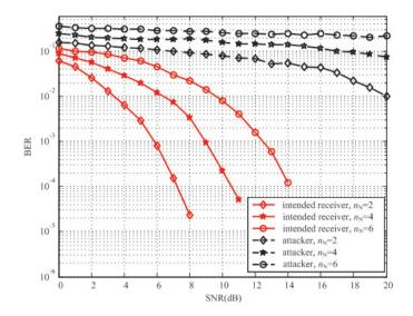
Figure 5: BER performance of novel MIMO secure communication system under fading channel, the noise sequences  $S_{noise}$  is secret
