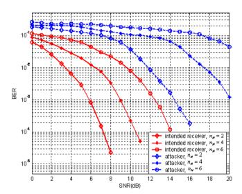
Figure 4: BER performance of novel MIMO secure communication system under fading channel, the noise sequences  $S_{noise}$  is public
