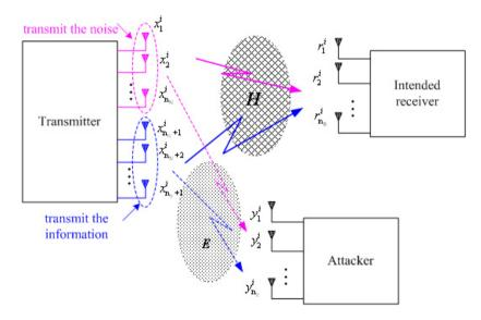
Figure 2: Antenna array redundancy model
