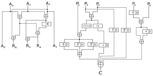
*Delay of the multiplier in*  $\mathbb{F}_4[X]$ . The critical path is made of the following three parts:
