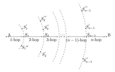
Figure 1: An *n*-hop Ad-hoc Network System for Information Exchange
