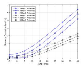
Figure 7: Secrecy Capacity Comparison between 2-hop and 3-hop under 2, 4 and 8 Antennas Equipment
