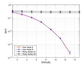
Figure 5: BER Performance Comparison between Different Nodes in 3-hop Information Exchange Protocol
